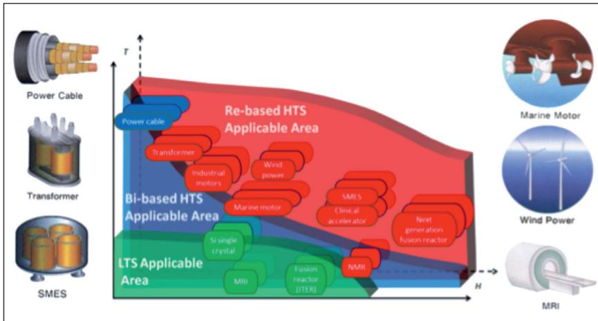
**FIGURE 5** Area of applications for LTS and HTS technologies with expected  $T$ - $H$  operation conditions
