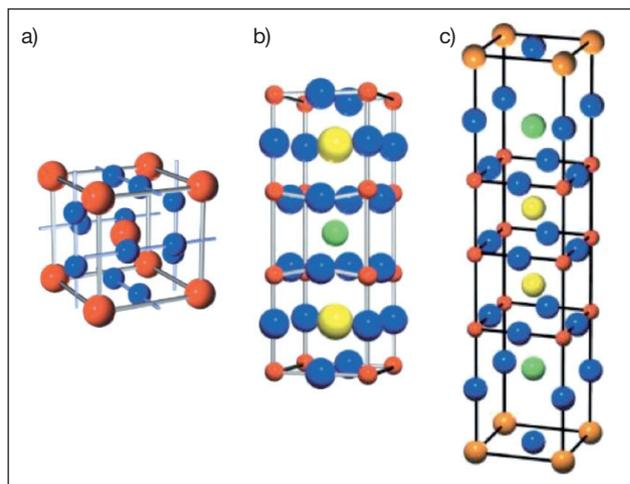
**FIGURE 2** Comparison among the crystal unit cells of different superconductors (not in scale): a)  $\text{Nb}_3\text{Sn}$ , cubic A15 structure; b)  $\text{YBa}_2\text{Cu}_3\text{O}_{7-x}$  orthorhombic perovskite; c)  $\text{Bi}_2\text{Sr}_2\text{Ca}_2\text{Cu}_2\text{O}_{10-x}$  tetragonal perovskite
