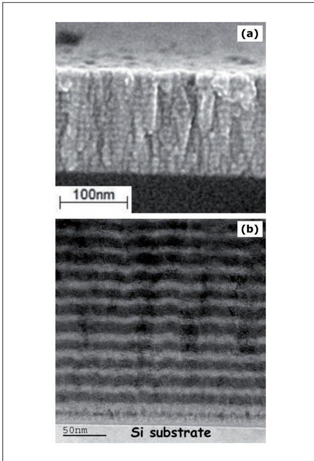
**FIGURE 3** (a) Cross-sectional FEG-SEM image of a ZrN/TiN multilayer coating with a bilayer period of 10 nm. (b) Cross-sectional high-resolution TEM image
