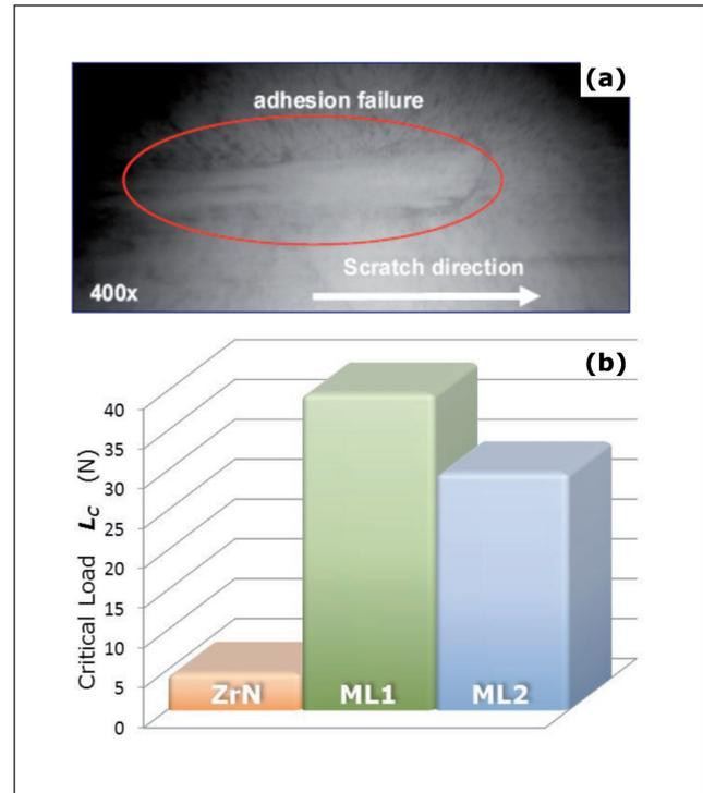
**FIGURE 4** (a) Optical microscope image of a scratch track on sample ML1. (b) Comparison of the critical load values for the different coatings
