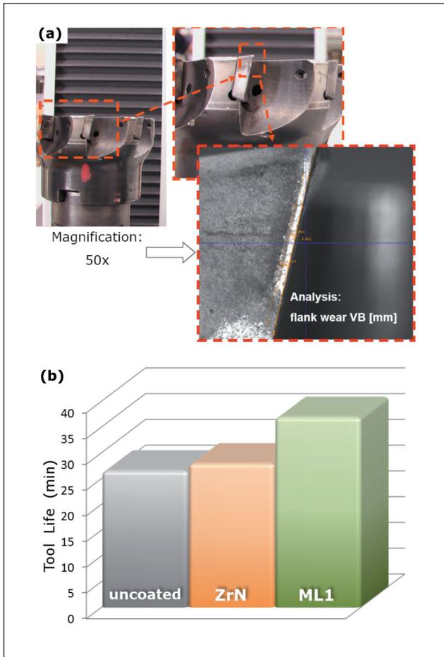
**FIGURE 5** (a) Detail of an insert mounted on a milling tool and magnification of the flank wear. (b) Comparison of tool life of uncoated inserts and inserts coated with a single ZrN coating and with a ZrN/TiN superlattice coating (ML1)
