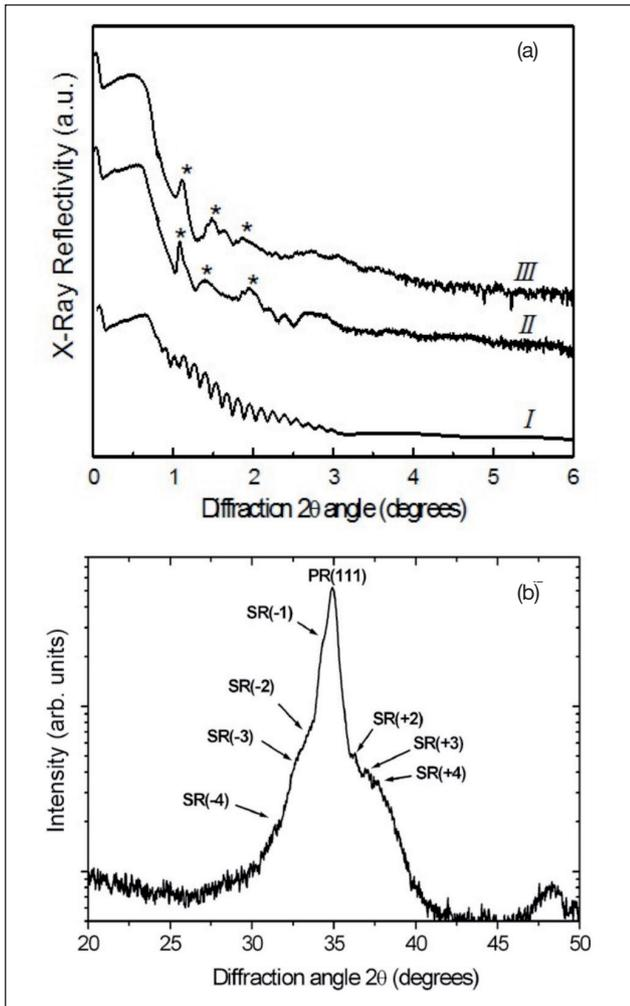
**FIGURE 2** (a) XRR spectra of three ZrN/TiN multilayers with bilayer period of about 2 nm (spectrum I), and about 8-11 nm (spectra II and III). (b) XRD spectrum of a multilayer sample with a 13 nm bilayer period
