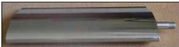
**FIGURA 6** Real-scale propeller profile coated with nanocomposite Ni deposit containing SiC NPs prepared at ENEA by laser pyrolysis
