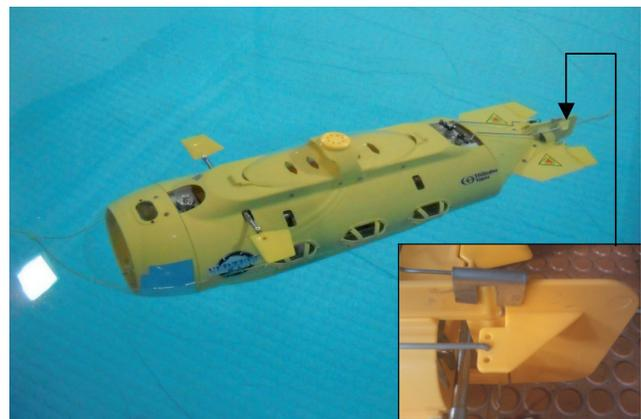
**FIGURA 1** Balance positioning to dive the submarine and lock the rudder system
