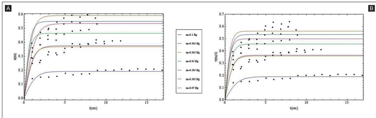
**FIGURA 4** A. Evolution of speed of weight as a function of its fall time with added mass - B. Evolution of the speed of weight as a function of its fall time without added mass
