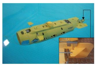
FIGURA 1 Balance positioning to dive the submarine and lock the rudder system
