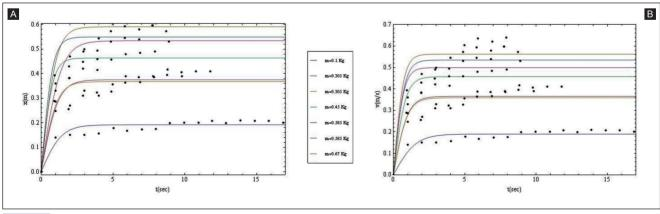
A. Evolution of speed of weight as a function of its fall time with added mass - B. Evolution of the speed of weight as a function of its fall time without added mass Source: ENEA
