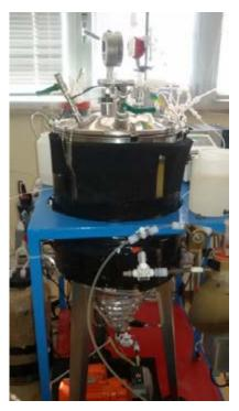
**Fig.4** A novel hybrid gas-stirred tank reactor (50L) treating dairy wastewater, implemented with a partial immobilization of the microbial community for in situ biomethanation research.
