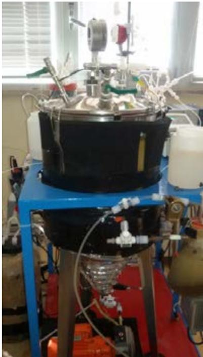
Fig.4 A novel hybrid gas-stirred tank reactor (SOL) treating dairy wastewater, implemented with a partial immobilization of the microbial community for in situ biomethanation research.
