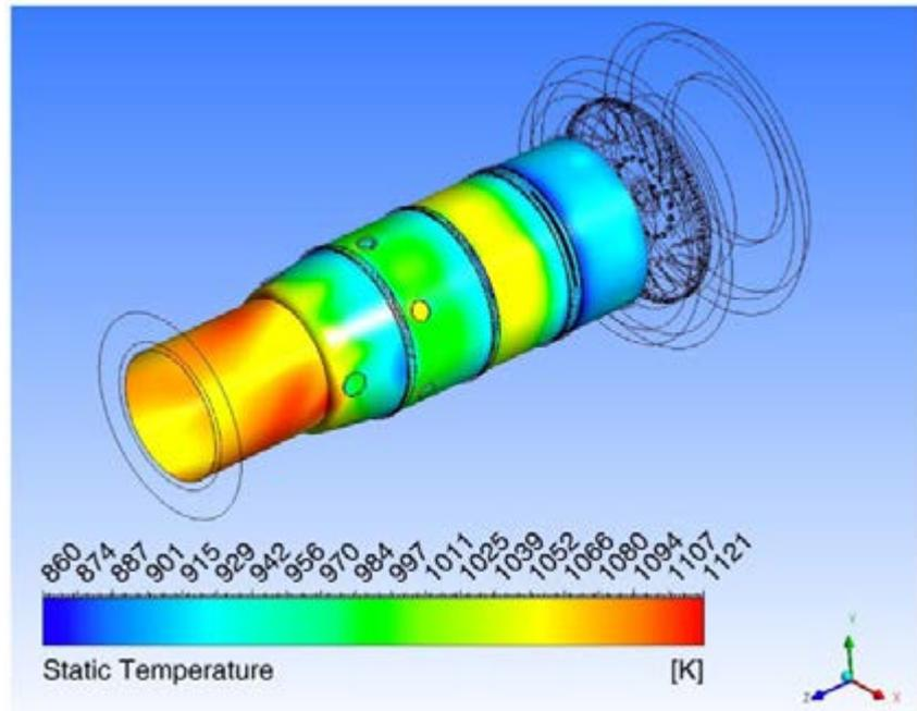
Fig.3 Temperature distribution on the liner inner walls of a micro-gas turbine combustor fed with methane and syngas [14].
