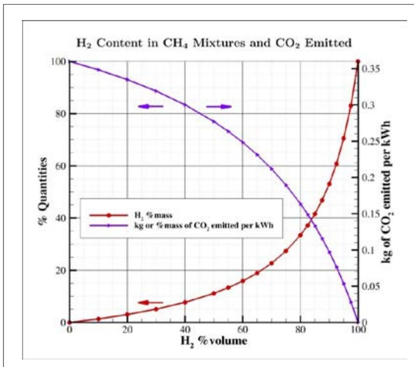
Fig.1 Relation between volume and mass percentages in methane/hydrogen mixtures, and impact in terms of CO<sub>2</sub> emitted (assuming an electrical efficiency of 55%). The percentage quantities on the left are with respect to pure methane.
