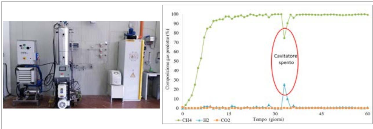
Fig.1 Hydrogenotrophic methanogenic reactor (1a - image on the left) and outlet gas composition (1b - chart on the right).
