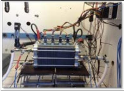
Fig.1 CNR ITAE-developed polymer electrolyte fuel cell stack prototype under laboratory testing.
