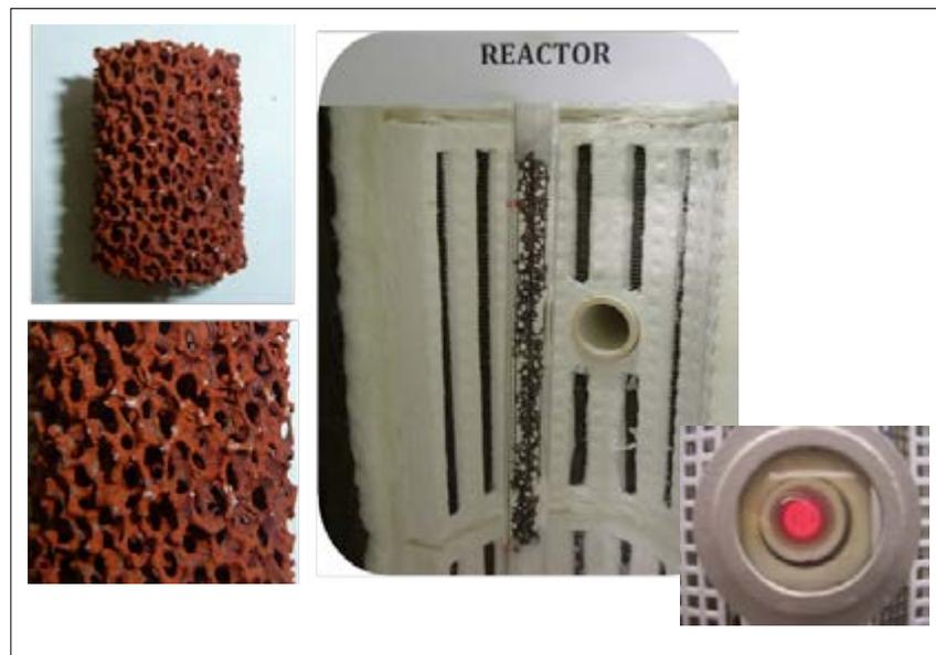
Fig.2 On the left, supported catalyst for SO<sub>3</sub> decomposition developed by ENEA within the SOL<sub>2</sub>Hy<sub>2</sub> European Project; in the center, catalyst sample placed inside the quartz lab reactor; on the right, catalyst in the quartz tube in operation during SO<sub>3</sub> splitting tests in the HycycleS European Project.
