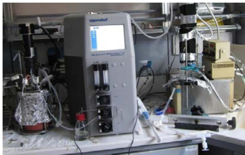
Fig.2 GRAIL project: 3L biofermenter collected to the gas-stripping apparatus for ethanol collection
