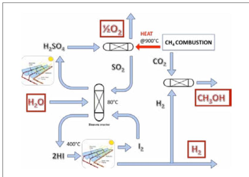
Fig.3 Alternative of the "Sulphur Iodine" scheme where H<sub>2</sub>SO<sub>4</sub> cracking is driven by methane combustion. The obtained CO<sub>2</sub> is reacted with part of the produced H<sub>2</sub> in order to synthesize methanol.
