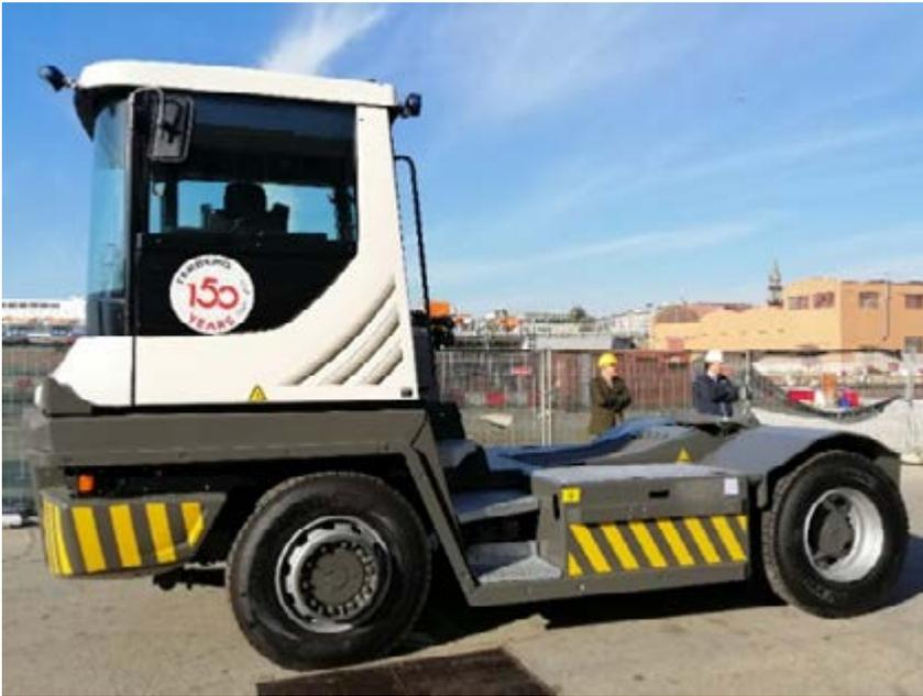
Fig.3 Yard Truck for port operation [3].
