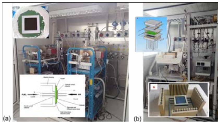
Fig.2 ABI laboratory test benches for SOC button cells in (a) and for single cells and short stack in (b)
