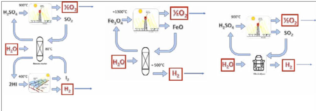
Fig.1 Three widely studied TWSCs: a) "Sulphur Iodine" b) "Iron Oxide" and c) "hybrid sulphur" cycles
