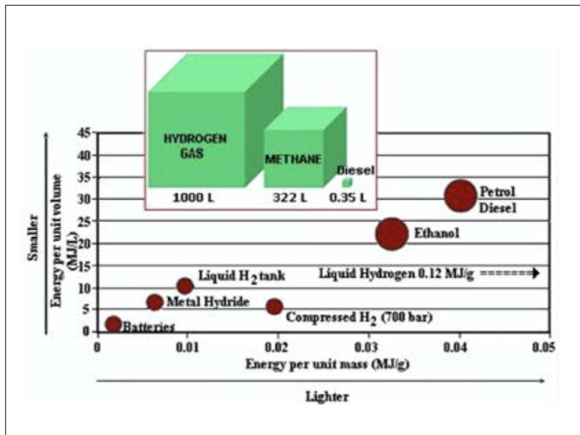
Fig.2 Energy densities of various energy storage materials and technologies, illustrating the respective volumetric and gravimetric densities [1]. The insert refers to volume gases at atmospheric pressure.
