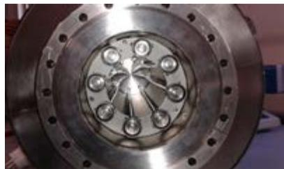
Fig.2 Scheme Internal view of a multi-tube membrane reactor for detritiation processes.
