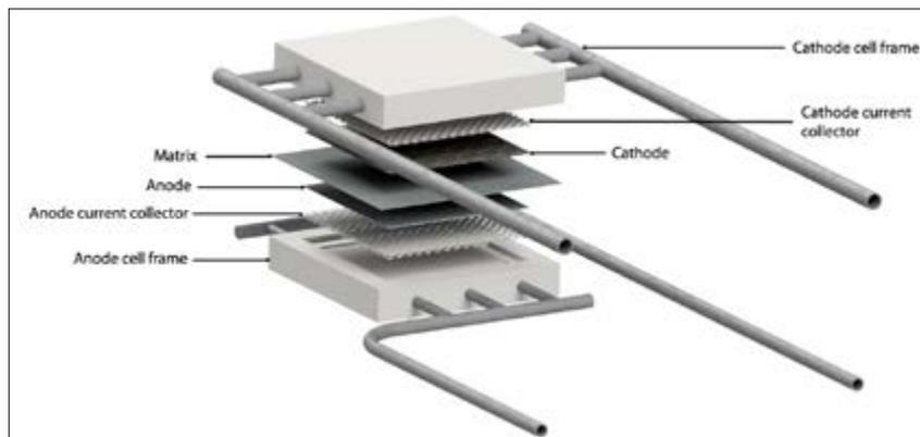
Fig.2 Working principles of MCFC/MCEC technology
