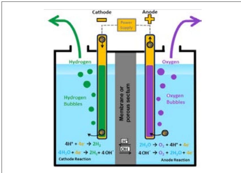
Fig.1 Simplified diagram of an electrolysis cell with alkaline or acid charge carrier.
