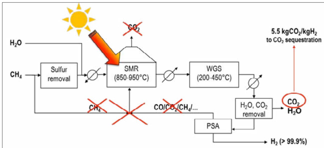
Fig.2 General scheme of a solar steam methane reforming process
