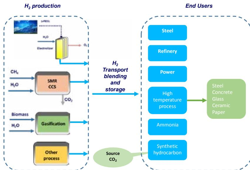
Fig.1 simplified scheme of hydrogen implementation in different industry sector
