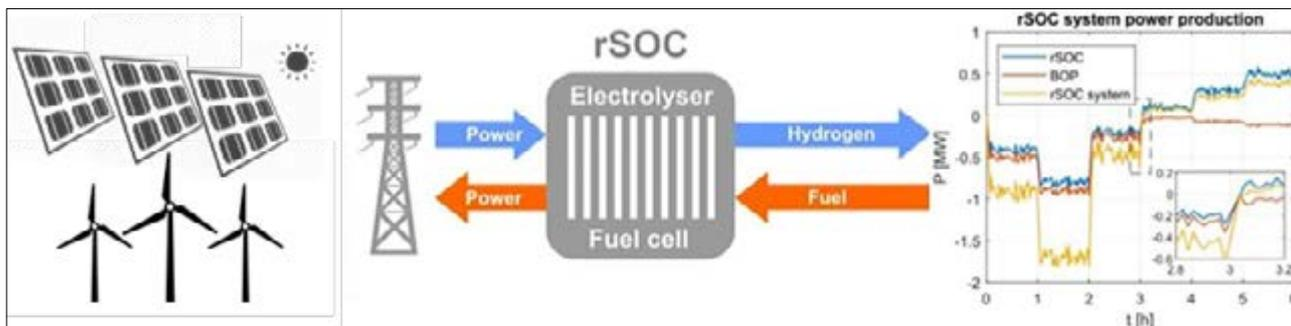
Fig.1 Simple schematic of an r-SOC system for RES balancing. (K. Motylinski et al. Energy Conversion & Management 228 (2021))
