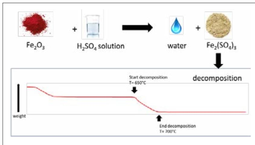
Fig.4 Alternative decomposition of sulfuric acid: the acid concentrated solution is reacted with Iron(III) oxide obtaining Iron(III) sulphate. The latter, as illustrated in the thermogravimetric pattern on the bottom, decomposes into Iron(III) oxide, sulphur oxides and oxygen at a lower temperature level than  $\text{H}_2\text{SO}_4$  itself (between  $650^\circ\text{C}$  and  $700^\circ\text{C}$ ).
