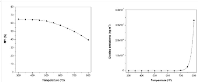
Fig.5 Methane yield (left) and dioxins emission (right) of a hydrogasification reactor fed with 1000 kg<sup>-1</sup> of dry RDF and a hydrogen excess of about 40 kg h<sup>-1</sup>. Reprinted from [18], with permission of Elsevier.
