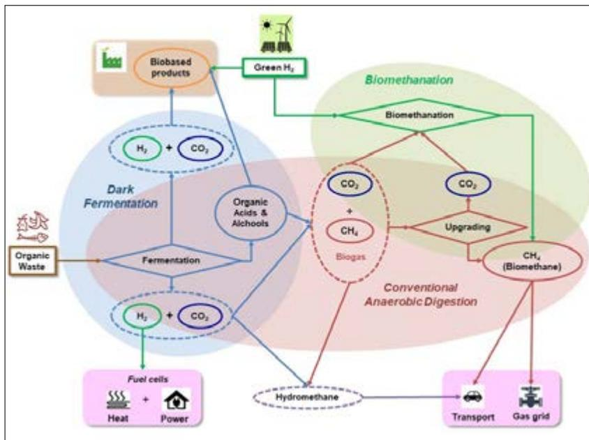
Fig.1 Biological processes integrated in the green H<sub>2</sub> value chain: Background coloured areas enclose the main step of each process; Rectangles represent process; feeding Diamond shapes represent technological stages; Round shapes represent products; Dotted lines enclose gas mixtures; Background coloured rectangles represent the end uses.
