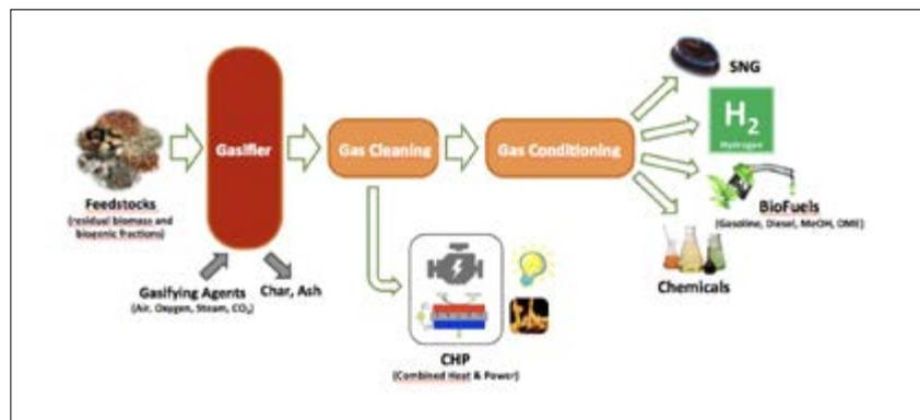
Fig.1 General process steps in gasification and related producer gas applications
