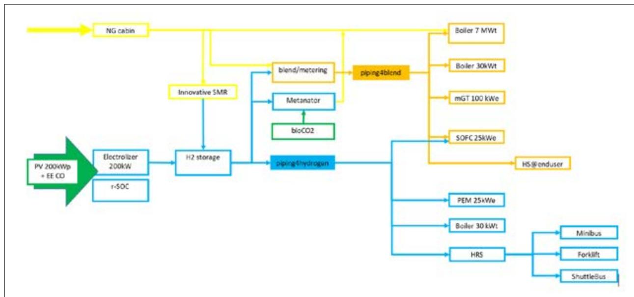
Fig.2 HV@ENEA Casaccia main process flow diagram
