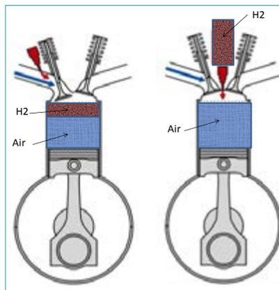
Fig.1 intake fuel injection and direct injection of H<sub>2</sub> in ICE
