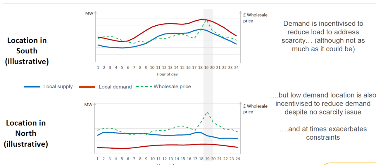
Figura 2: The single national price is creating inaccurate signals for demand to respond
