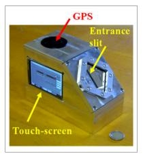
Fig. 4 The solar compass designed for parabolic trough mirror driving
