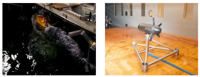
Fig. 2 Left: 1.5 m diameter model turbine during wave/current interaction tests in the wave tank (Courtesy Schottel Hydro GmbH); Rigth: Two 0.4 m model turbines during simulated turbine operation in array in the Circulating Water Channel (Courtesy SABELLA SAS)
