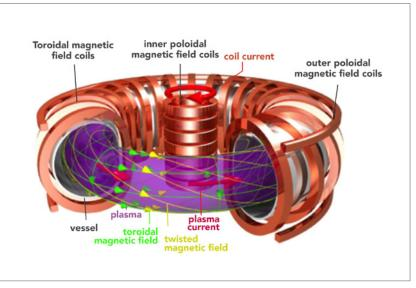
Fig. 1 Schematic view of magnetic confinement in a Tokamak
