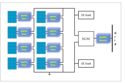
Fig. 2 SMPPC Master-Slave architecture
