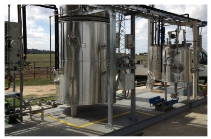
Fig. 3 Two-stage anaerobic digestion pilot plant at CREA Research Centre in Monterotondo
