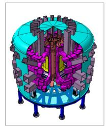
Fig. 3 Sectional view of DTT tokamak basic machine
