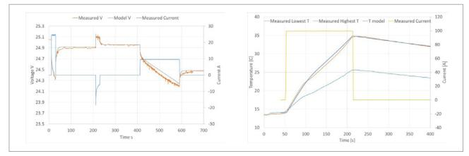
Fig. 3 Comparison between measured and calculated voltages during the test to measure the internal resistances of the module (left); Discharge at 20C current with forced convection and gas speed at 20 m/s (right)
