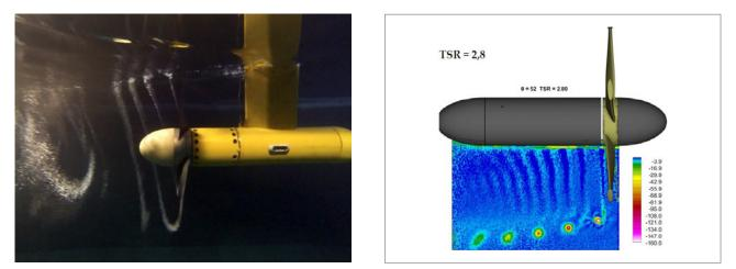
Fig. 1 Left: Air entrained by the tip vortex of a 1.5 m diameter model turbine during towing tank test; Right: Vorticity distribution in the wake of a SABELLA model turbine from PIV measurements in the Circulating Water Channel [2]
