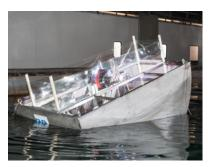
Fig. 6 PEWEC 1:12 prototype during test operations in the towing tank in Rome
