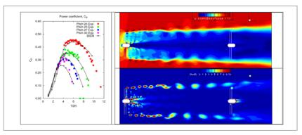
Fig. 3 Left: Turbine performance predictions by BIEM, power coefficient predictions for different blade pitch settings [3]; Right: Computational study by Hybrid RANS/BIEM model of flow around two coaxial turbines spaced d = 4 diameters. Instant axial velocity (top) and vorticity intensity
