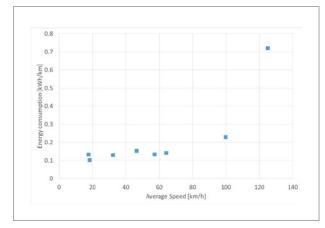
Fig. 5 Influence of the average speed on consumption for HIZEV electric
