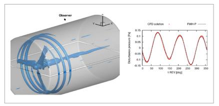
Fig. 5 Left panel: FWH-P surface and vortices core detection; right panel: Acoustic pressure near field
