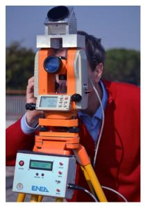
Fig. 2 The ENEA electronic solar compass mounted on a theodolite
