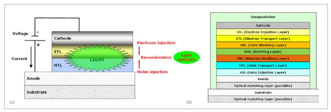
Fig. 1 (a) Basic OLED structure and working mechanism: usually the electron transport layer is also the emitting layer. (b) Example of OLED structure aimed at increasing the performances
