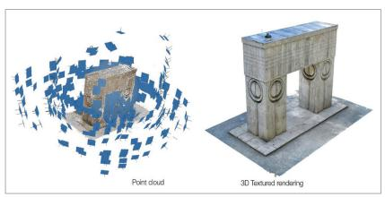
Fig. 2 Digital backbone - detailed photogrammetry model
