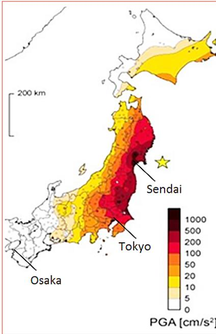
**FIGURE 1** Peak ground acceleration recorded at the 2011 Great East Japan Earthquake
