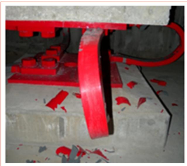
**PHOTO 2** Deformation of U-shaped steel damper
