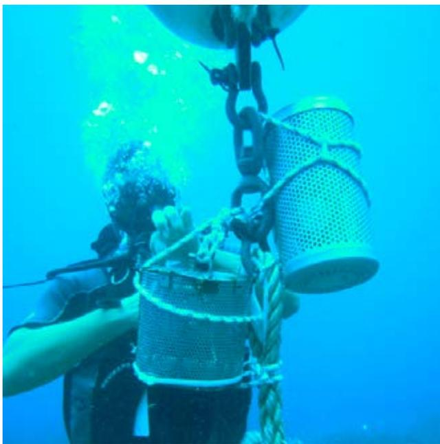
**FIGURE 3** Passive sampler placement by scuba diver in Preveto site
