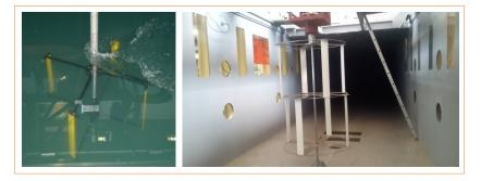
FIGURE 4 Examples of vertical-axis marine current turbines (VACT) models tested in the CNR-INSEAN towing tank (Kobold turbine, left), and flume tank (ABENGOA project, right)
