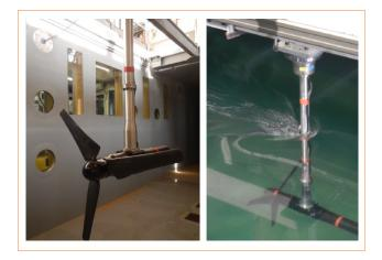
FIGURE 6 The horizontal-axis, 3-bladed rotor designed at IFREMER (France) used in the Round-Robin tests. Pictures show trials at CNR-INSEAN water flume (left) and towing tank (right)
