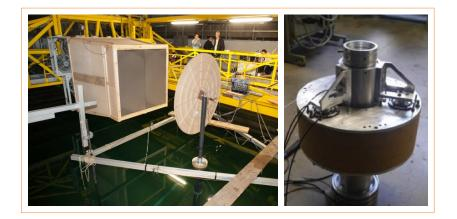
FIGURE 8 Wave tank tests at CNR-INSEAN of the STC system, a hybrid wave/wind energy device. Overview of the set-up with wind generators and nozzle (left) and close-up of the WEC (right)
