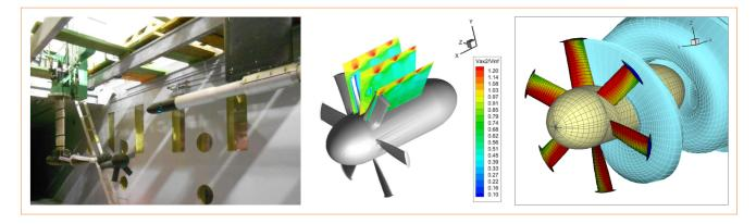
FIGURE 5 SABELLA horizonthal-axis turbine: set-up in the CNR-INSEAN water flume (left), results of wake flow measurements by Laser-Doppler velocimetry (center) and results of CFD simulations (right)
