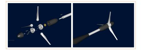
FIGURE 2 CAD model of a three-bladed model turbine built for tests in the flume tank
