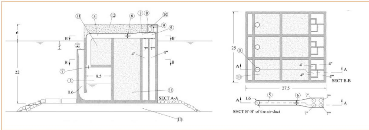
**FIGURE 3** Example of REWEC2. 1 air pocket; 2 outer opening; 3 air feed; 4 air reservoir; 5 air duct; 6 Wells turbine; 7 butterfly valve; 8 service room; 9 exhaust valve; 10 compressor; 11 sand filling; 12 superstructure cast in concrete; 13 rubble mound foundation; volumes of reservoirs: 4I, 55 m<sup>3</sup>; 4II, 110 m<sup>3</sup>; 4III, 220 m<sup>3</sup>; 4IV, 275 m<sup>3</sup>
