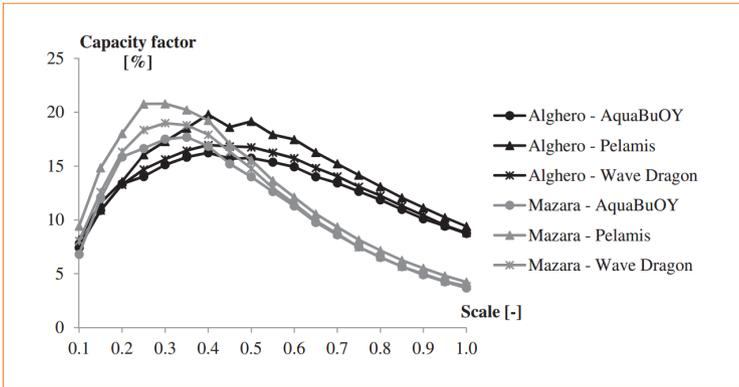
**FIGURE 1** Capacity factors at Alghero and Mazara for different device dimensions
