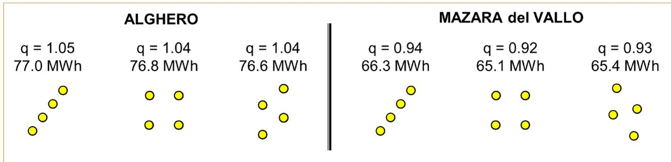
**FIGURE 10** Optimal array configurations at the study sites
