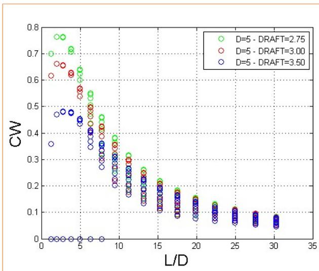
**FIGURE 3** Capture width vs. L/D (L wave Length, D cylinder diameter) for the most efficient cylindrical buoy
