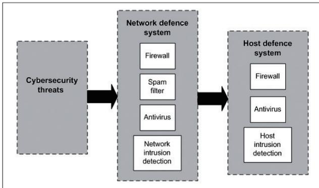
**FIGURE 3** A typical cyber security protection system
