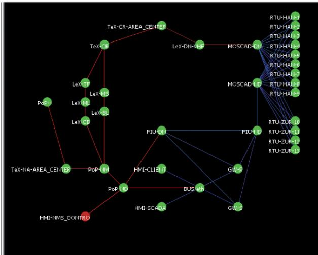
**FIGURE 4** The infection starts on an NMS device of corporate network
