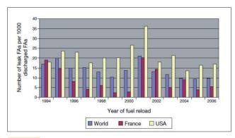
FIGURE 3 IAEA figures on FA found fault with leaks after inspection Source: IAEA
