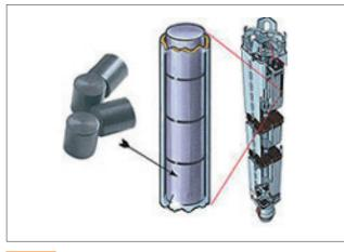
FIGURE 2 From fuel pellets to rods and assembly Source: http://www.skb.se
