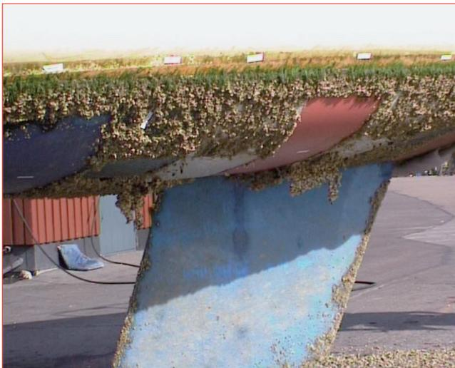
**FIGURE 2** Example of fouled ship hull
