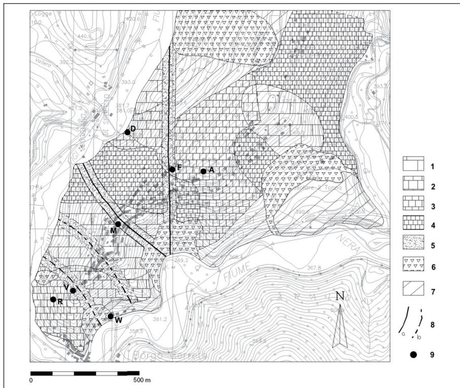
**FIGURE 4** Map of rock mass classes: 1) moderately jointed rock mass (Class A); 2) highly jointed rock mass (Class B); 3) intensely jointed rock mass (Class C); 4) very intensely jointed rock mass (Class D); 5) rock mass from intensely jointed to mylonitic, lying astride each fault (Class E); 6) slope and landslide debris; 7) not classified rock mass; 8) certain (a) and uncertain (b) fault; 9) velocimetric station
