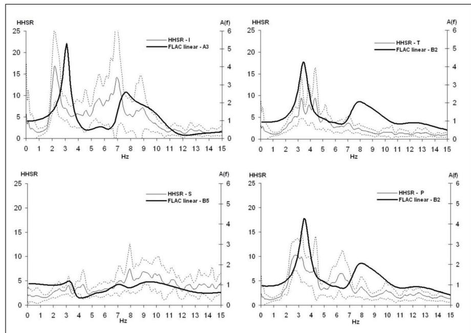
**FIGURE 5** Comparison between SSRs  $\pm$  standard deviation (dashed lines) from weak motions and 2D numerically modelled  $A(f)$ , for the velocimetric stations I, T, S and P (see Fig.2 for location)
