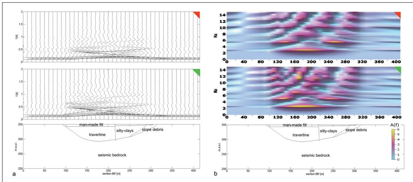
**FIGURE 6** S<sub>w</sub> wave propagation (a) and A(f) function (b) resulting by the 2D numerical modelling along section BB' of Fig.2, for both homogeneous (red right corner) and heterogeneous (green right corner) conditions
