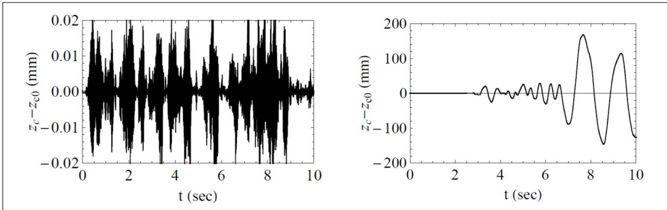
**FIGURE 12** Horizontal displacement of the centre of gravity due to: a) Seismic acceleration following the Italian code; b) Seismic acceleration amplified by a factor 4
