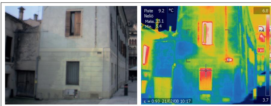
**FIGURE 10** Moisture distribution and moisture growth detected by thermal scanning
