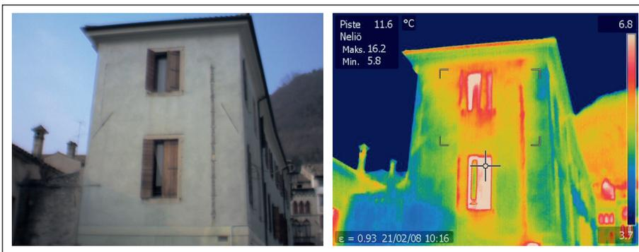
**FIGURE 9** Thermal image applied to detect discontinuities beneath the surface, using an inclusive range among 3.7° and 6.8° for the thermographs staircase. It is possible to see a different superficial temperature of materials for that heated places internally
