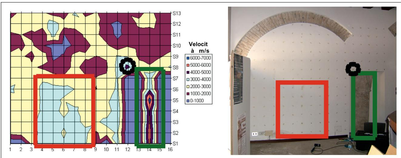
**FIGURE 6** Distribution of the pulse sonic velocity on the wall
