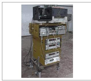
FIGURE 1 RGB-ITR scan system in tower configuration. Lasers and electronic units are allocated in the yellow boxes, while the optical head is above Source: ENEA
