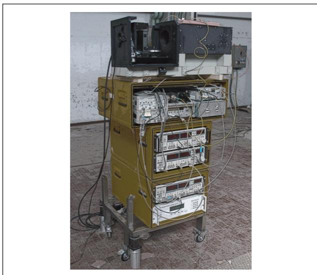
**FIGURE 1** RGB-ITR scan system in tower configuration. Lasers and electronic units are allocated in the yellow boxes, while the optical head is above
