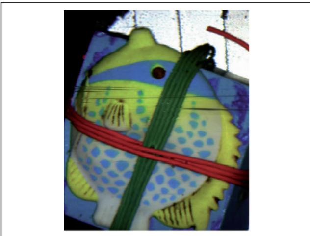
**FIGURE 5** Result obtained by an upgrade of the RE-VUE system equipped with three CW AM laser sources at 450nm (blue,  $f_m=100\text{MHz}$ ), 532nm (green,  $f_m=30\text{kHz}$ ) and 650nm (red,  $f_m=190\text{MHz}$ ): high-resolution and high-contrast 3D color image of a plastic fish immersed in a 2m-high clean water column acquired at high rate (1000 sample points per second)
