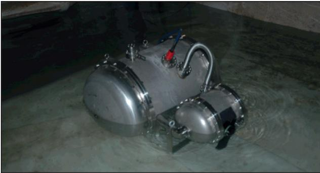
**FIGURE 4** Photo of the RE-VUE system used for underwater 3D imaging. The small cylinder contains the laser source, the scanning system and the receiving stage (lens and fast photomultiplier). The big cylinder, instead, hosts the electronic modules (e.g., lock-in amplifier)
