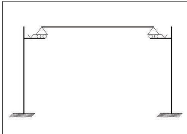
**FIGURE 8** Scheme of the simply supported beams with friction
