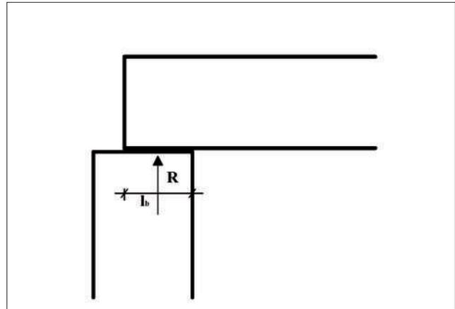
**FIGURE 3** Schematic representation of the column-beam interface
