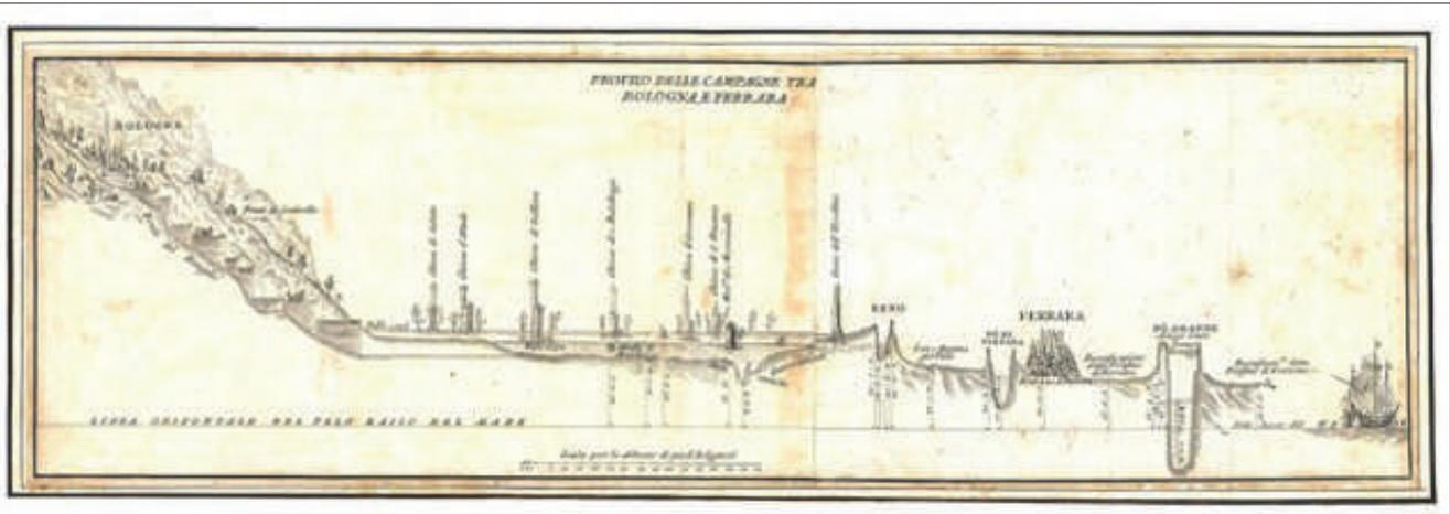
**FIGURE 1** Sketch summarizing the details of Reno River deviation, started in 1604, as was proposed by Giovanni Domenico Cassini. The profile extends from Bologna (left) to Ferrara (right)
