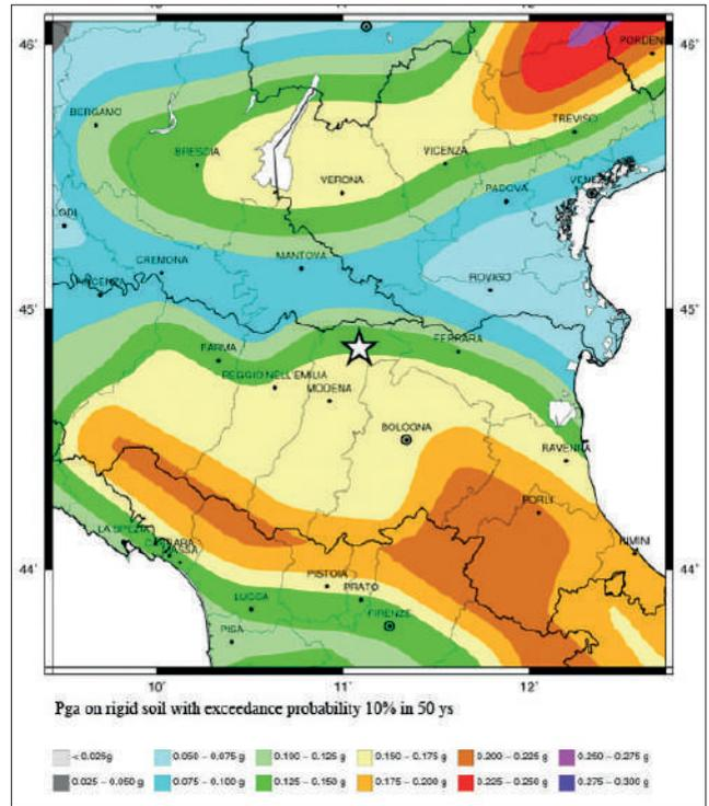
**FIGURE 8** Design basis PGAs
