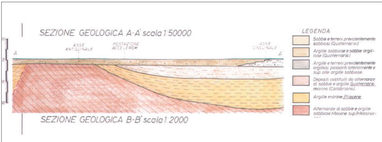
**FIGURE 13** Mirandola station geological cross section
