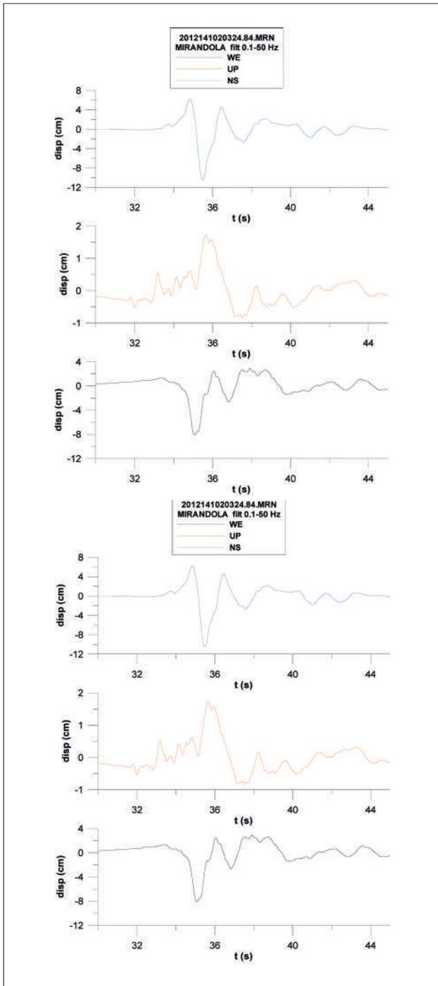
**FIGURE 1** Displacement time-histories recorded at Mirandola (A) and Modena (B)
