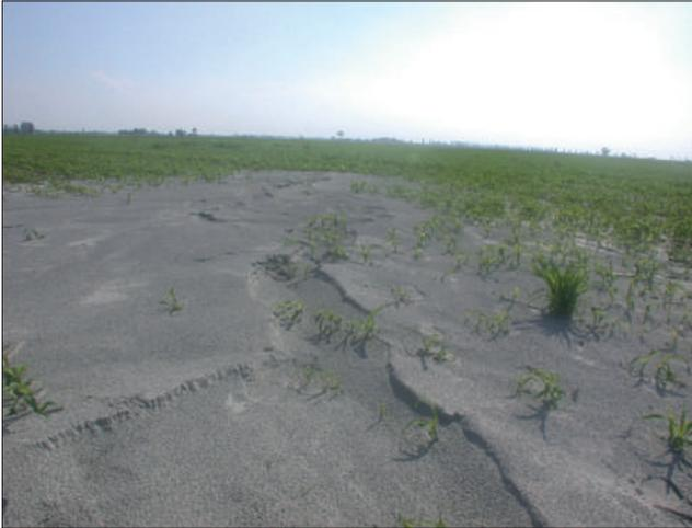
**FIGURE 9** Soil liquefaction near Bondeno
