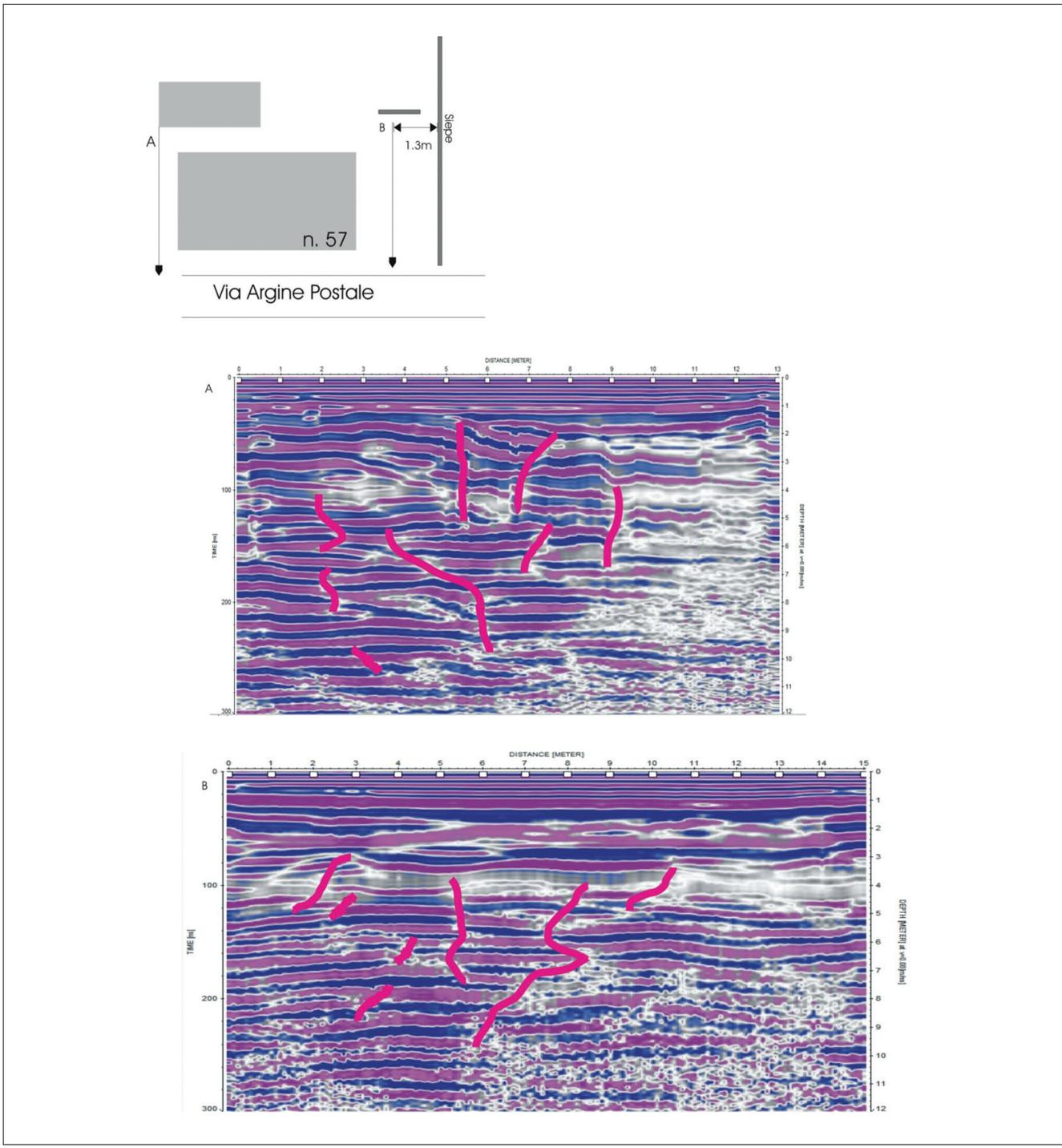
**FIGURE 5** Example of GPR sections, 100 MHz, recorded on the side of building in via Argine Postale 57 at Mirabello. Possible fractures and/or sand intrusions are highlighted in red. The upper left insert shows the position of the GPR and seismic profiles with respect to the building. A and B: GPR sections. Thick vertical line: seismic reflection profile
