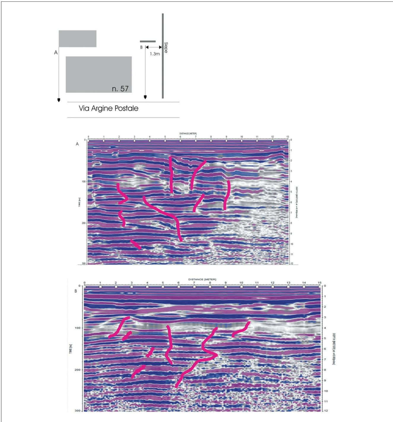
**FIGURE 5** Example of GPR sections, 100 MHz, recorded on the side of building in via Argine Postale 57 at Mirabello. Possible fractures and/or sand intrusions are highlighted in red. The upper left insert shows the position of the GPR and seismic profiles with respect to the building. A and B: GPR sections. Thick vertical line: seismic reflection profile
