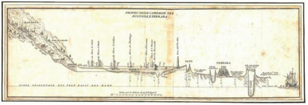
**FIGURE 1** Sketch summarizing the details of Reno River deviation, started in 1604, as was proposed by Giovanni Domenico Cassini. The profile extends from Bologna (left) to Ferrara (right)
