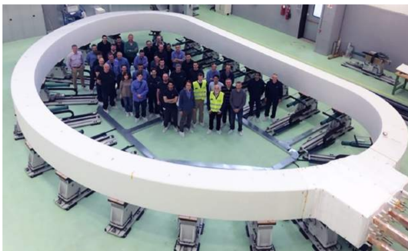
Fig. 4 The first-ever Winding Pack for the Toroidal Field coils Source: courtesy of ASG Superconductors, La Spezia, Italy
