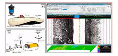
FIGURE 3 Main resources used for hydrographic surveys. a) Multibeam and sidescan sonar transducer with dynamic motion sensor. b) Marine DGPS dual antenna for position and heading. c) Example of multibeam echo sounder and sidescan sonar data acquisition during survey operations
