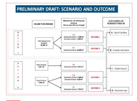
FIGURE 8 Schematic flow diagram which describes the possible options of contamination, subsequent dredging volume and management scenarios
