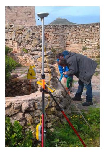
FIGURE 5 Measuring the DGPS position and elevation
