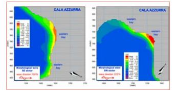
FIGURE 19 Simulation of mean surface elevation induced by morphological waves at Cala Azzurra
