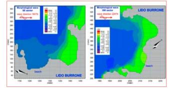
FIGURE 20 Simulation of mean surface elevation induced by morphological waves at Lido Burrone
