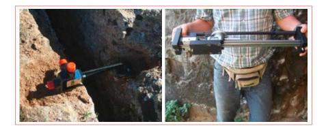
FIGURE 3 3D joint meter installed on the giant joint of the plateaux of the west side of Cala Rossa (left) and the removable deformeter during the measurement survey
