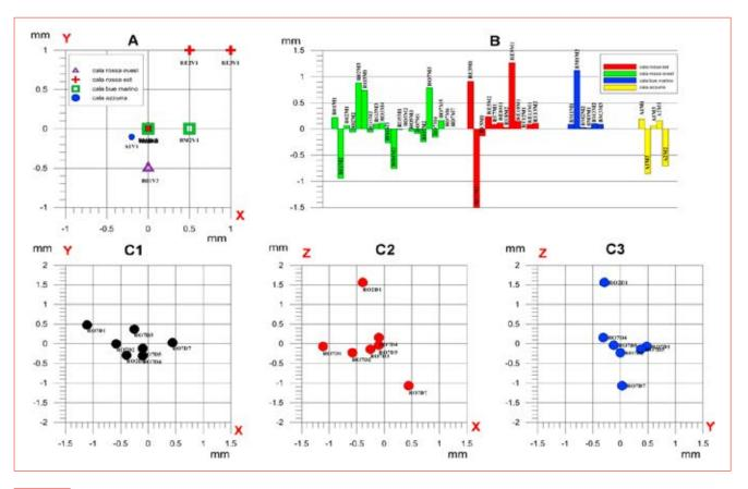
FIGURE 10 Displacements measured with the mechanical joints gauges: tell tales (A), removable joint-meters (B) and 3D joint-meters (C1, C2 and C3)
