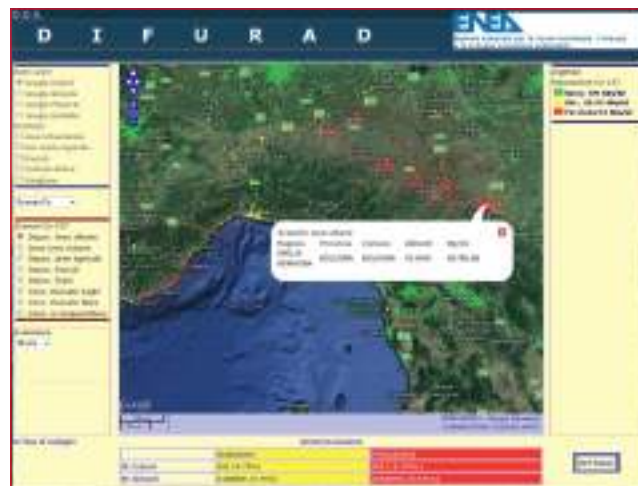
FIGURE 6 Example of Scenario: ^{137}\text{Cs} cumulated ground deposition ( \text{Bq}/\text{m}^2 ) over Urban Areas. In the lower part of the WebGIS application it also possible to access detailed reports
