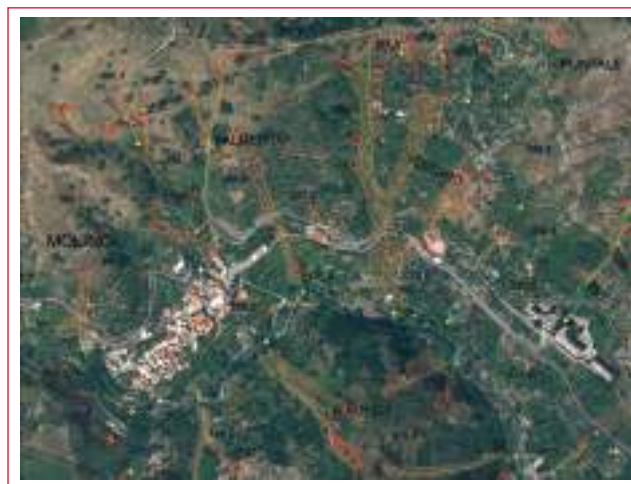
FIGURE 2 Example of the georeferenced features of some debris-mud flows contained in the inventory (red triangle: triggering point; yellow dot: stop point; red line: triggering area; orange hatched: transport and depositional area; green line: run out path)
