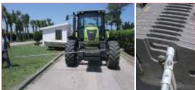
FIGURE 3 Fledging bar installed on a tractor of the Di Vaira farm. Right: detail of the bar hook
