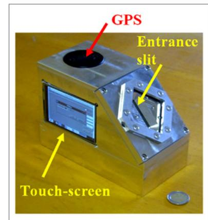
Fig. 4 The solar compass designed for parabolic trough mirror driving
