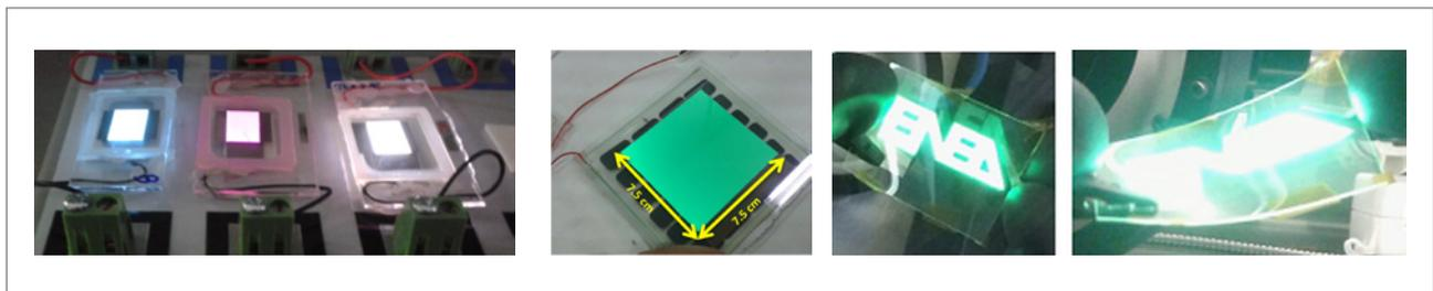
Fig. 2 ENEA NANO OLEDs: (a) on glass, area 1 cm<sup>2</sup> and about 55 cm<sup>2</sup>; (b) on plastic
