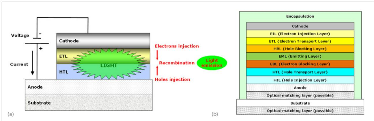
Fig. 1 (a) Basic OLED structure and working mechanism: usually the electron transport layer is also the emitting layer. (b) Example of OLED structure aimed at increasing the performances
