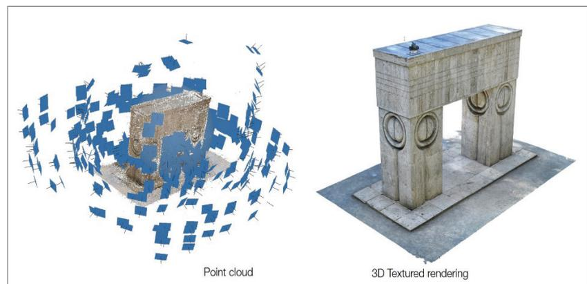
Fig. 2 Digital backbone - detailed photogrammetry model
