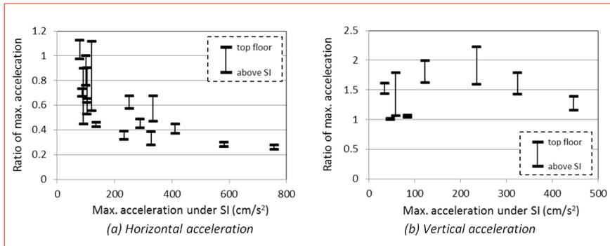
**FIGURE 5** Maximum acceleration ratio of superstructure to foundation
