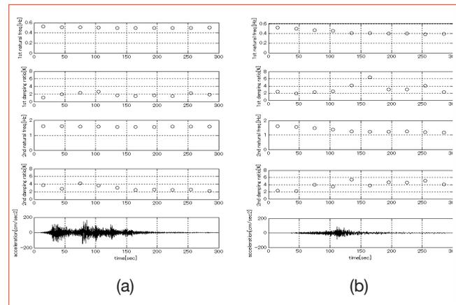
**FIGURE 9** Change of vibration characteristics of high-rise buildings during the earthquake (Saito 2012). (a) Steel building in Sendai (H1 direction); (b) Reinforced concrete building in Tokyo (H1 direction)
