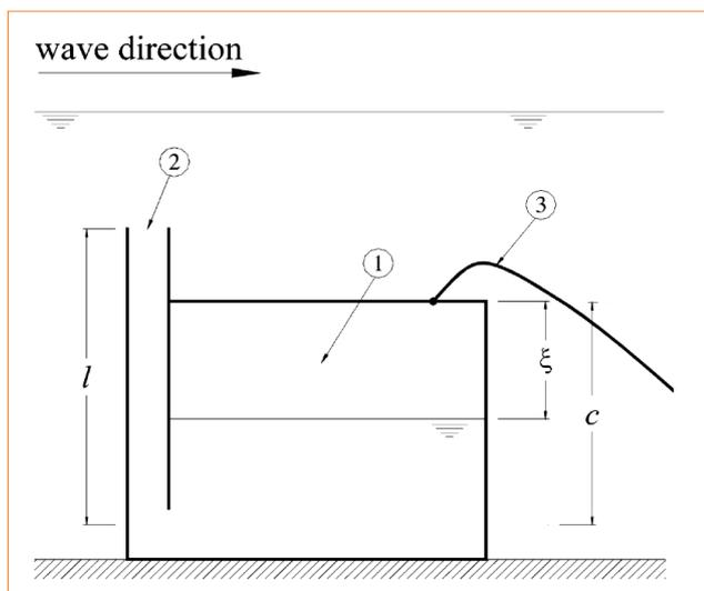
**FIGURE 2** Scheme of a REWEC including an air pocket (1), a vertical duct (2) and an air feed (3)
