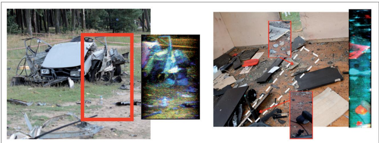
**FIGURE 9** Fluorescence images of areas of the outdoor (left) and indoor (right) scenarios reconstructed by the RGB method
