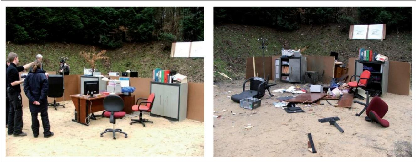
**FIGURE 6** Scenario in Bièvres test before (left) and after (right) the blast
