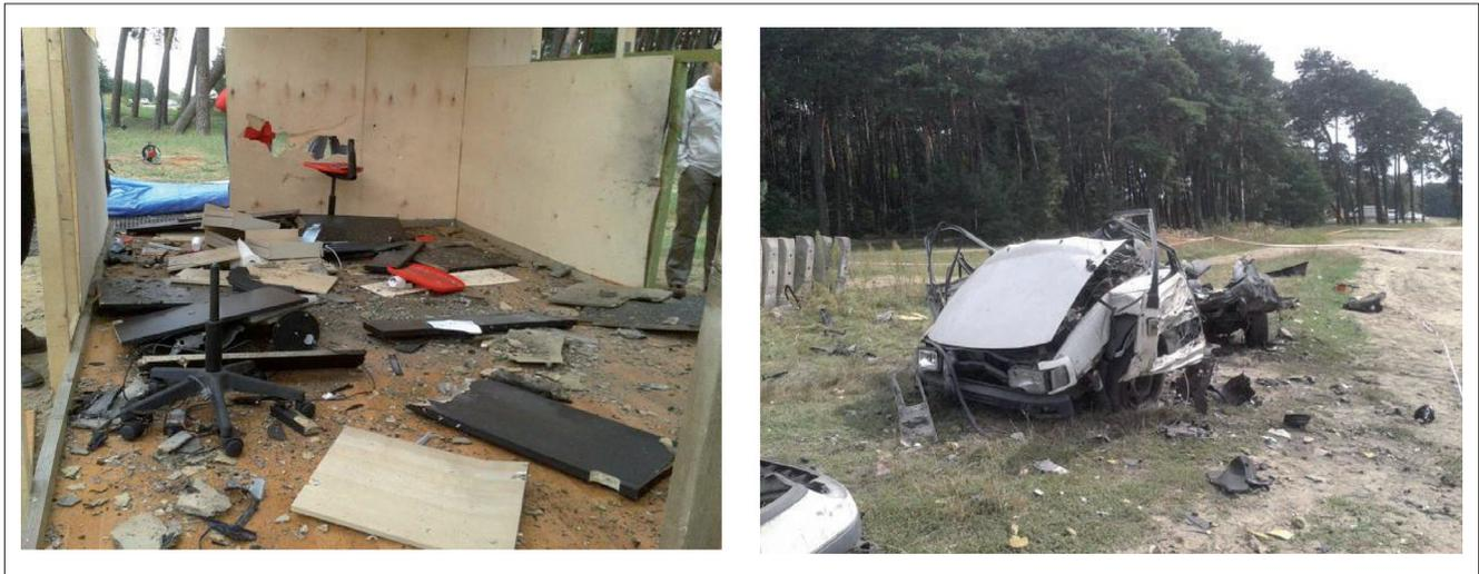
**FIGURE 8** Post-blast outdoor and indoor scenarios in Wrocław's test
