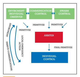
FIGURE 10 Principle control scheme
