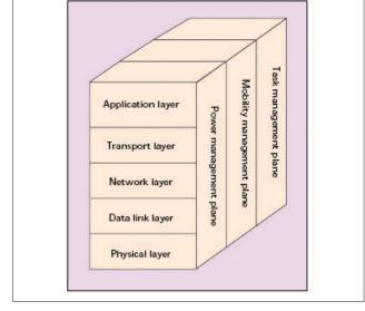
FIGURE 9 Protocol Stack for Harness project
