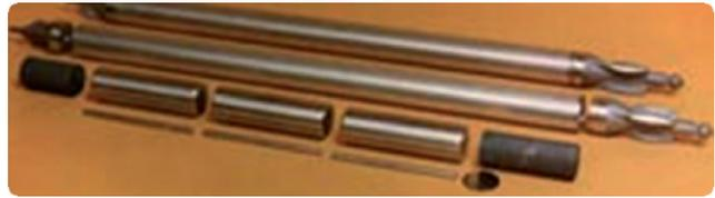
**FIGURE 5** The TRIGA Fuel Rods
