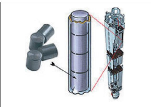
**FIGURE 2** From fuel pellets to rods and assembly
