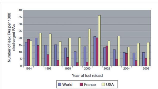
**FIGURE 3** IAEA figures on FA found fault with leaks after inspection
