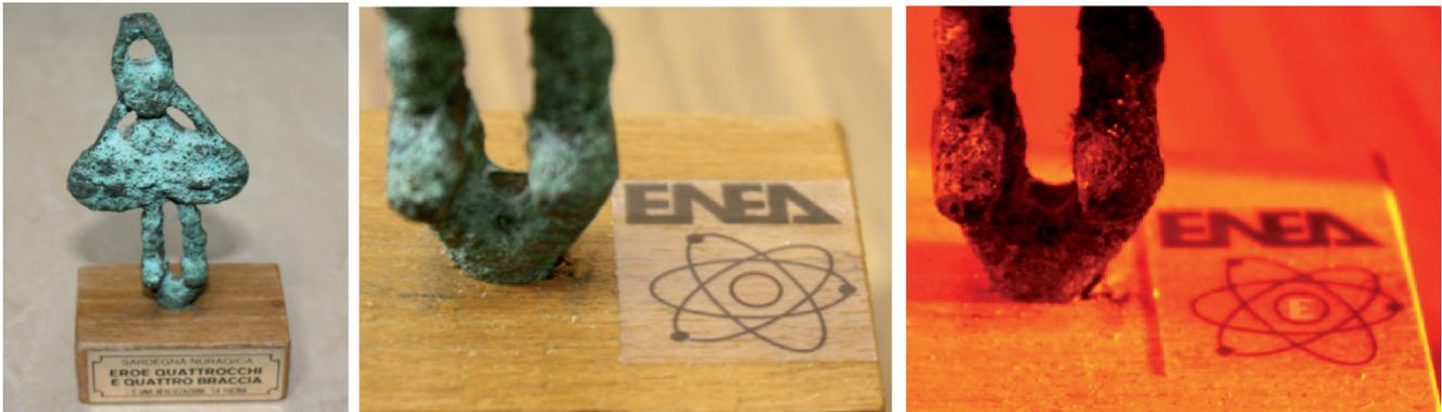
**FIGURE 2** Left: Copy of an archaeological bronze statue, known as “hero four-eyes and four-arms”, height: 11 cm; Middle: The transparent and adhesive tag based on a LiF film stuck on the wood base of the statue; Right: The letter ‘E’ patterned by EUV radiation appears when using the patented reading technique
