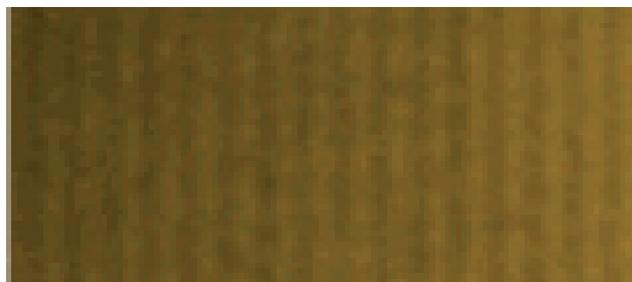
**FIGURE 1** Luminescent patterns stored on a LiF film deposited by thermal evaporation on a glass substrate at ENEA [8], obtained by the MET-EGERIA described in [4, 5]. The pattern period is 2.2 micrometers
