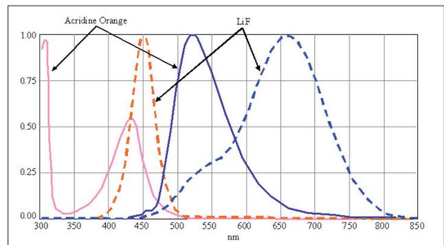
**FIGURE 3** Optical absorption and emission spectra of LiF colour centres (dashed lines) and of Acridine orange (continuous lines) in the range 300 nm - 850 nm. Acridine orange is one of the dyes having the most similar absorption and emission spectra vs. LiF
