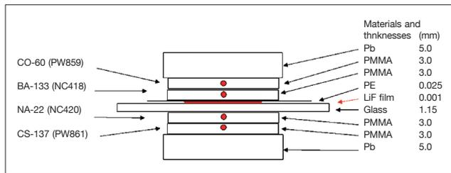
**FIGURE 4** Schematic of the irradiation setup of the LiF film patterned with the invisible EUV-marking. The film was sandwiched between several radio-nuclides and exposed to a total dose of 1,700 Gy during 40 days of continuous exposure
