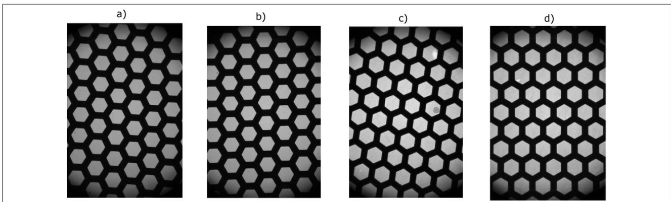
**FIGURE 5** Microscope views of the invisible pattern on the LiF films evidenced by the patented reading technique. The period of the hexagonal pattern is about 0.05 mm. From left to right: a) Before irradiation; b) After 40 days of irradiation with a total dose of 1700 Gy; c) Reference sample, not irradiated; d) The same reference sample after 40 days
