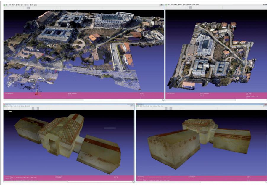
**FIGURE 2** Example of a UAV-derived cloud with 108 mil. points with related RGB colour loaded remotely using Meshlab (a). A textured polygonal model with 3 mil. polygons and ca 115 MB texture displayed within Meshlab (b)
