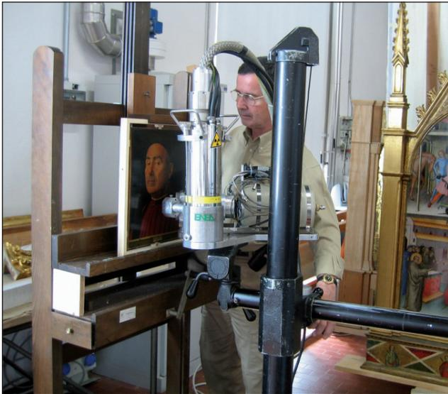
**FIGURE 1** The Trivulzio portrait during the execution of the XRF measurements
