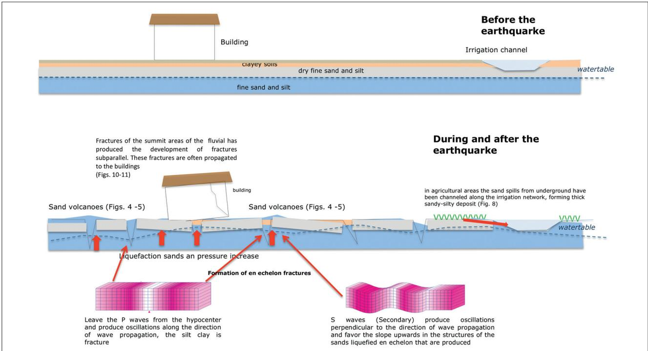
**FIGURE 9** Soil liquefaction and effects on the stability of man-made structures: up) before the earthquake; low) during and after the earthquake
